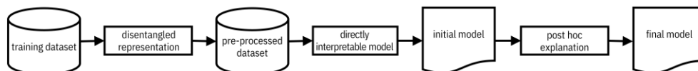
Figure 12.3. Pipeline view of explanation methods. Accessible caption. A block diagram with a training dataset as input to a disentangled representation block with a pre-processed dataset as output. The pre-processed dataset is input to a directly interpretable model block with an initial model as output. The initial model is input to a post hoc explanation block with a final model as output.
