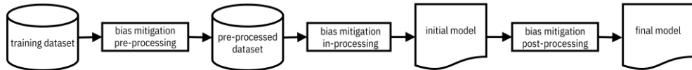
Figure 10.8. Three types of bias mitigation algorithms in different parts of the machine learning pipeline. Accessible caption. A block diagram with a training dataset as input to a bias mitigation pre-processing block with a pre-processed dataset as output. The pre-processed dataset is input to a bias mitigation in-processing block with an initial model as output. The initial model is input to a bias mitigation post-processing block with a final model as output.
